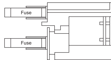
Fuse installation for 220/240 voltage
