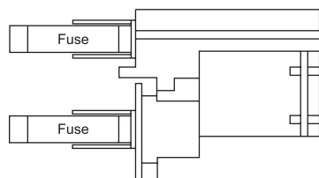
Fuse drawer for 220/240 voltage selection
